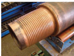
Too little thread compound
